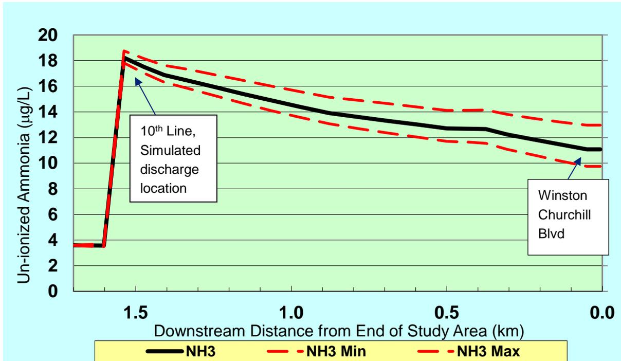
Figure 14. Full Build Out: Un-ionized Ammonia in the West Credit River Predicted by QUAL2K for Low Summer flow and 0.7 mg/L Effluent TAN
