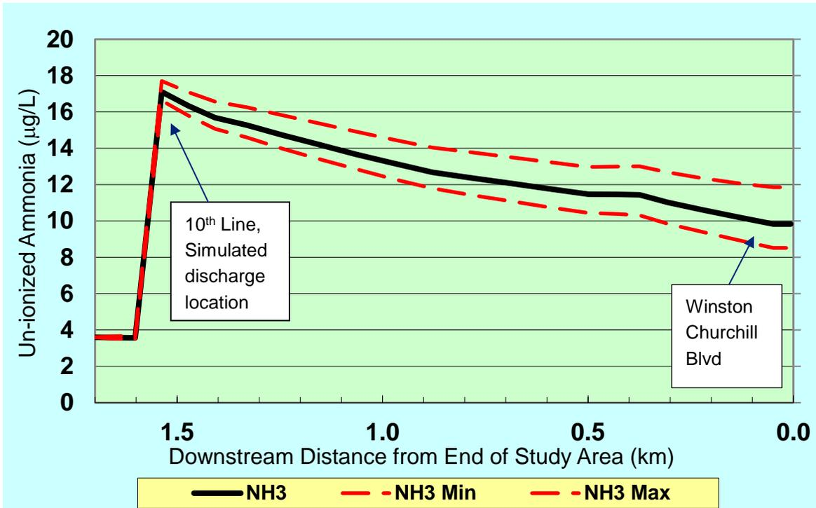
**Figure 13. Phase 1: Un-ionized Ammonia in the West Credit River Predicted by QUAL2K for Low Summer flow and 1.3 mg/L Effluent TAN**
